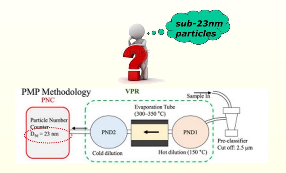
To properly define a measurement procedure for sub-23 nm particles emitted from internal combustion engines it has to be better understood their nature.
