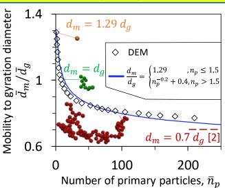
The ratio of mean mobility diameter over that of gyration,  $\bar{d}_m/\bar{d}_a$ , evolves from 1.29 for single spheres, but rapidly decreases to 1 for agglomerates with  $n_p \sim 10$  and asymptotically reaches 0.7 (dashed line) for large agglomerates with  $\bar{n}_p \ge 700$  [2]. The DEM-derived relation [3] (solid line) quantifies the evolution of  $\bar{d}_m/\bar{d}_g$  within 4% of DEM simulations.
