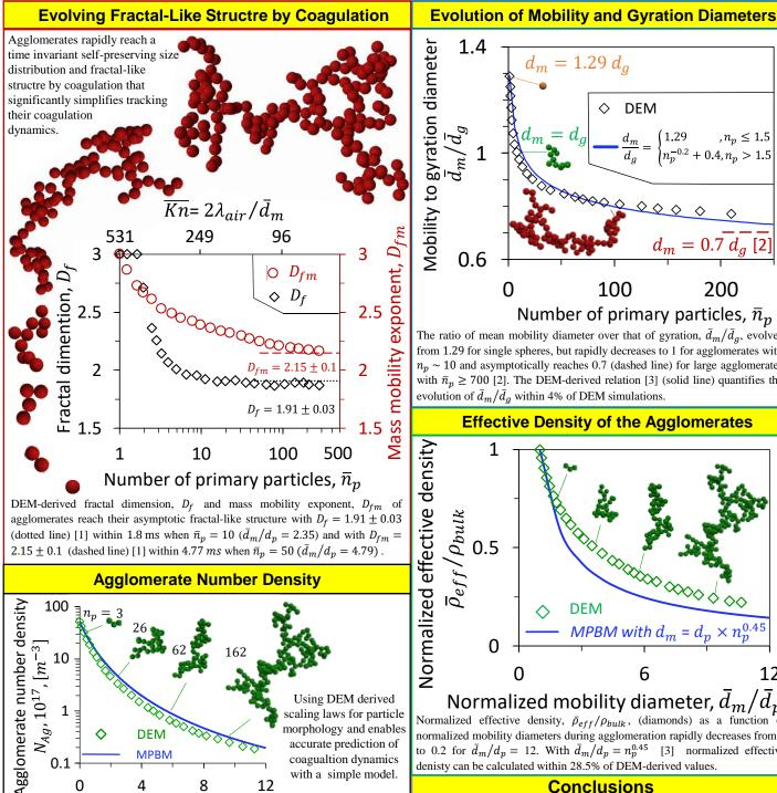
**Time** [ms] Evolution of a)  $N_{Ag}$  and b)  $\bar{n}_p$  as a function of time during agglomeration in the free molecular regime derived by DEM (diamonds) and MPBM (lines) simulations.
