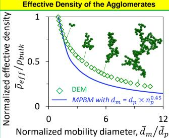
Normalized effective density,  $\bar{\rho}_{eff}/\rho_{bulk}$ , (diamonds) as a function of normalized mobility diameters during agglomeration rapidly decreases from 1 to 0.2 for  $\bar{d}_m/d_p = 12$ . With  $\bar{d}_m/d_p = n_p^{0.45}$  [3] normalized effective denisty can be calculated within 28.5% of DEM-derived values.
