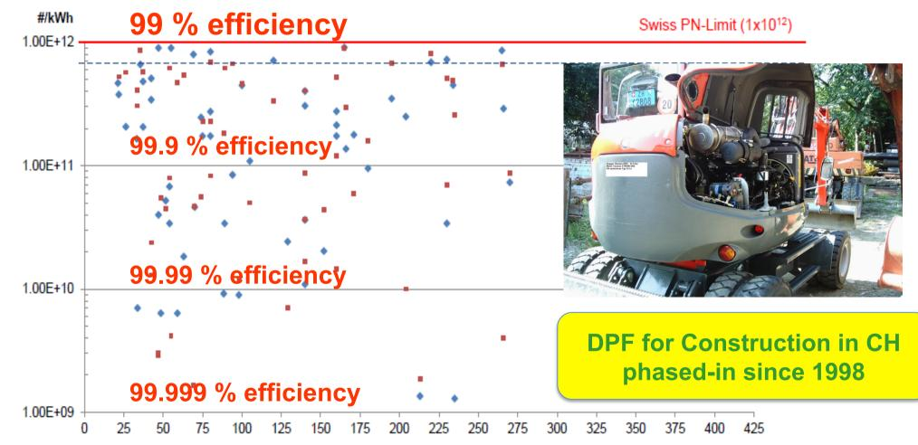
Type approval of imported construction machines in stationary and transient cycle In function of engine power [kW]
