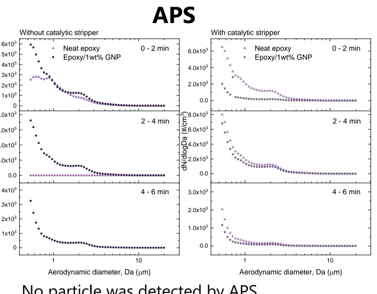
No particle was detected by APS after 6 minutes.
