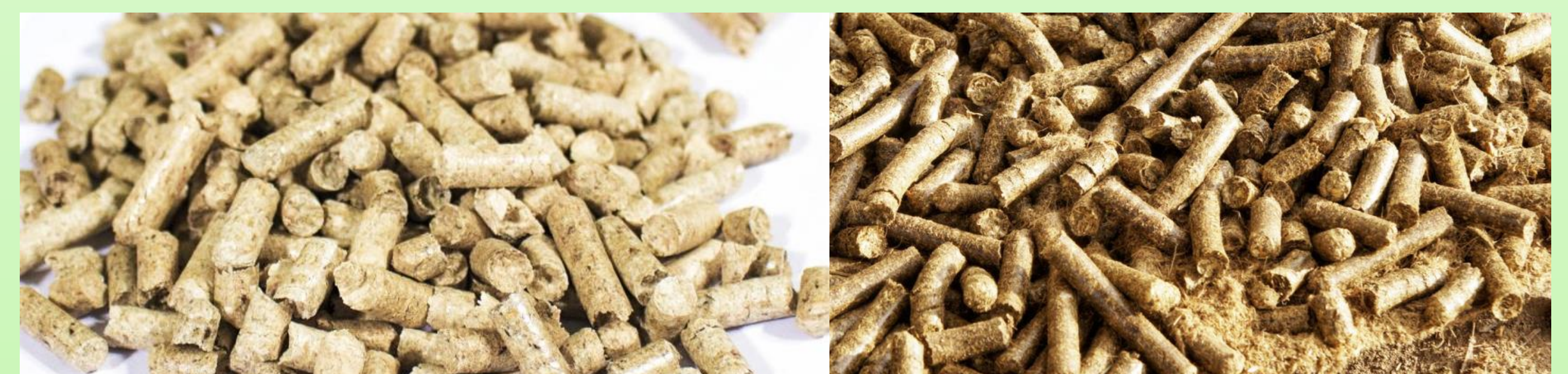
Fig. 4 The Spruce-pellets (left) and the agro-pellets were formed from waste agricultural biomass (right)
