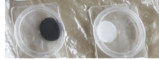
Quartz filter with black carbon for particle phase on the left and filter for gas phase on the right before sampling
