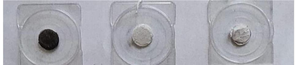
Particle phase after CAST for different combustion conditions
