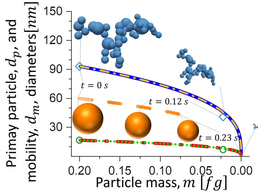
Neglecting soot fractal-like structure results in significant error in predicting its coagulation & oxidation rates
