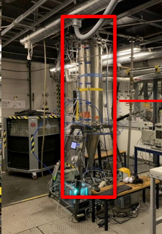
Experimental setups at the ILMARI-laboratory: A SKODA SCALA vehicle on a chassis dynamometer in connection with the high-volume PEAR oxidation flow reactor
