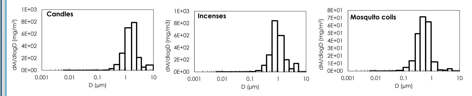
• The combustion of **candles**, **incenses** and **mosquito coils** is responsible for the emission of airborne particles, especially in the sub-metric range ( $D_p < 1\mu m$ ). The chemical analyses conducted with ELPI impactor show the presence of different hazardous chemical compounds;
