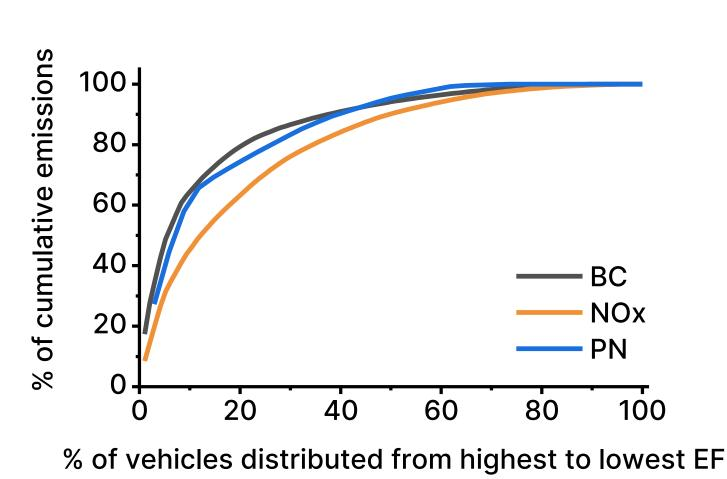
10% of vehicles with highest EF in 2023 sample contribute 65% of BC and PN emissions, and 46% of NO<sub>x</sub> emissions.
