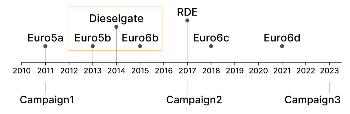
The on-road chasing method is an independent real-world vehicle emission testing method, where emissions of random, in-use vehicles are measured by chasing them on the road. We analyzed EF distributions from 3 on-road chasing measurement campaigns to evaluate the effectives of the legislation aimed to reduce emissions of on-road vehicles.
