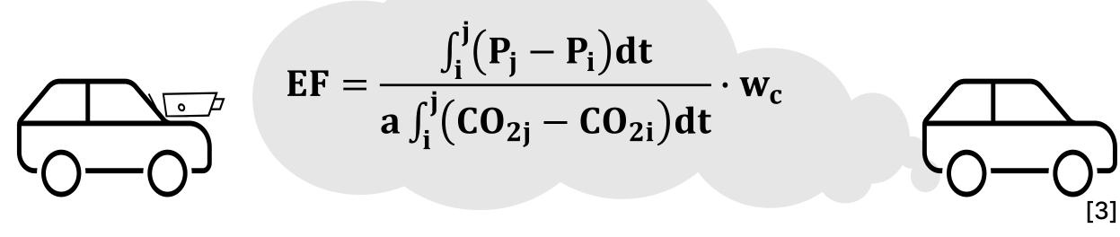
P = BC, PN or Nox, a = 0.2727, w<sub>c</sub> is 0.86. Instruments: CO2 – Carbocap GMP 343, BC – Aethalometer AE33, NOx - 2B Technologies 410 and 401 (2011), EcoPhysics, CLD86 (2017), and AL2 (2023); PN - TSI, FMPS (2011 & 2017) and CPC (2023).
