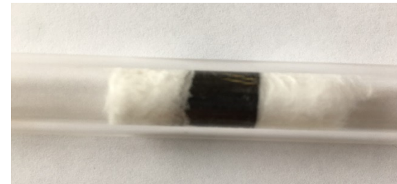
Reactor with Mn 2 O 3 /soot blend
