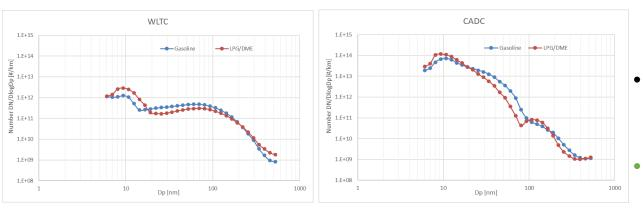
High speeds -----> production of ultrafine particles (< 10 nm) ٠ in both cycles and for both Gasoline and LPG/DME
