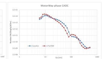
Low speeds ----> production of slightly bigger particles (> 30 nm) in the WLTC cycle for both Gasoline and LPG/DME
