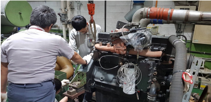
Engine mounted on dynamometer
