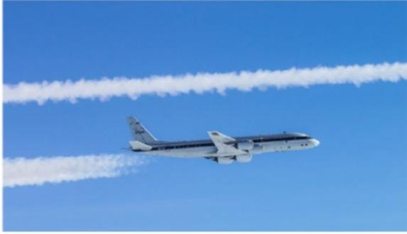
Fig. 1 The NASA DC8 research aircraft probing contrails from the DLR A320 burning a sustainable aviation fuel blend above Germany
