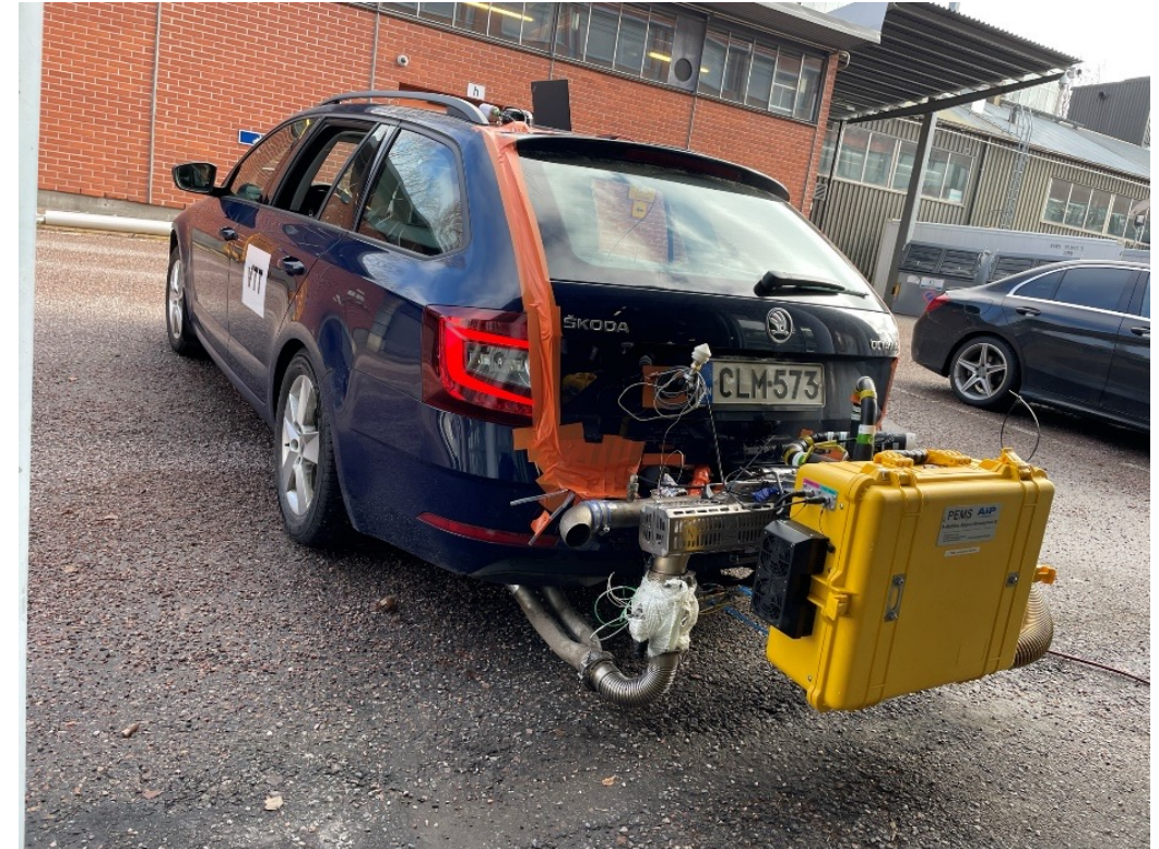
Skoda Octavia gasoline with two PEMS systems installed before RDE test
