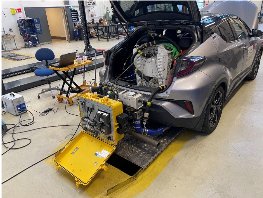
Toyota C-HR gasoline hybrid with two PEMS systems installed on chassis dyno
